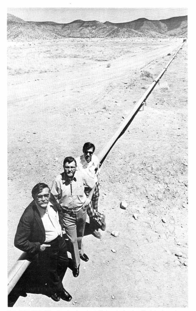
MILE-LONG VACUUM PIPE encloses laser beam, heart of the largest and most sensitive strain seismometer ever designed, operating in Coyote Canyon. From left are Ben Benjamin (1123), Wendell Weart (1140) and Doug Gabin (1111).
